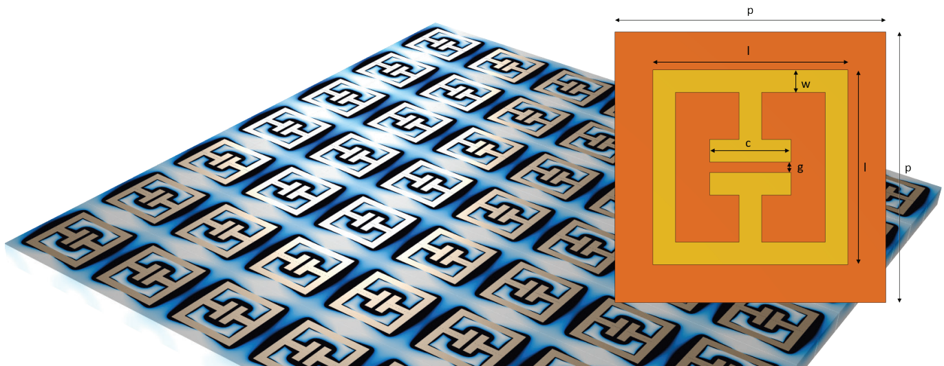
FIGURE 3 The simulation results for a terahertz absorber structure (left) show the magnitude of the electric field. The unit cell of the absorber (right) has a 200-nm layer of gold on an 8- \mu\text{m} polyimide substrate. The polyimide is backed by a continuous ground plane of gold (not shown). Cell dimensions: p = 36 \mu\text{m} , l = 25.9 \mu\text{m} , w = 3 \mu\text{m} , c = 10.8 \mu\text{m} , and g = 1.4 \mu\text{m} . See Reference 2.
