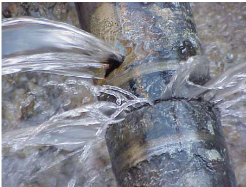
FIGURE 1. Left: Leaky pipe under investigation. Right: Schematic of leak detection setup. A leak is bracketed by two sensors whose distance is D . The leak sound propagates in both directions and a correlator measures the time it takes to reach each sensor. Based on the speed of sound in the pipes, the exact leak location can be found.
