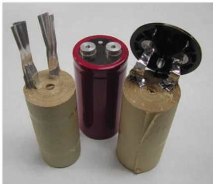
FIGURE 1. Aluminum electrolytic capacitors. The windings are composed of aluminum foils and cellulosic separators, and exhibit thermal anisotropy.
