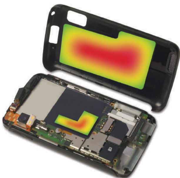
Figure 5. Flexible graphite foil heat spreaders enable dissipation of heat from an electronic component with high in-plane conductivity, while protecting underlying heat-sensitive areas with low through-plane conductivity. Photo courtesy of GrafTech International.
