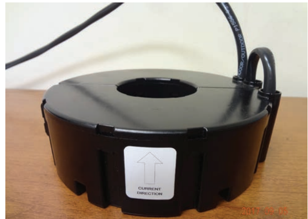
Figure 6. The submersible split-core sensor.
