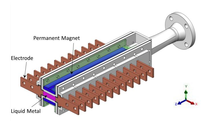
Figure 3: MHD generator with cross-section cut-out view along the x-y plane
