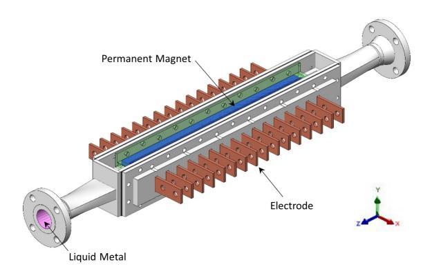
Figure 1 : Assembly drawing of the MHD generator
