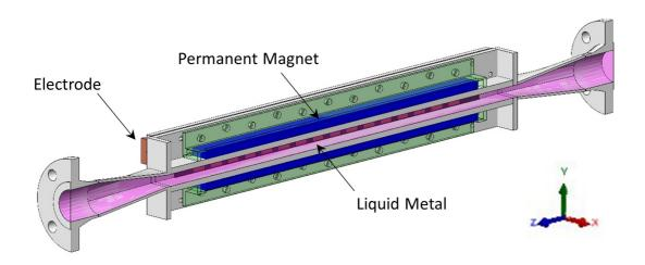
Figure 2: MHD generator 3D view with cut-out section along the y-z plane
