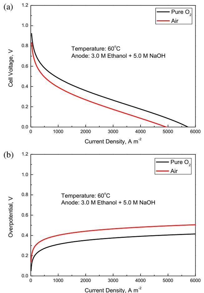
**Fig. 8 – Effect of the oxygen concentration on the cell performance. (a) Polarization curves; (b) Cathode overpotentials.**
