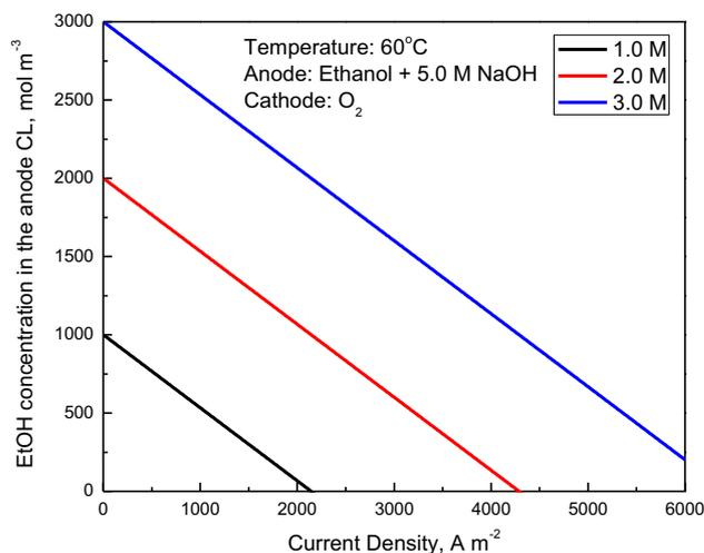
**Fig. 5 – The ethanol concentration in the anode CL.**
