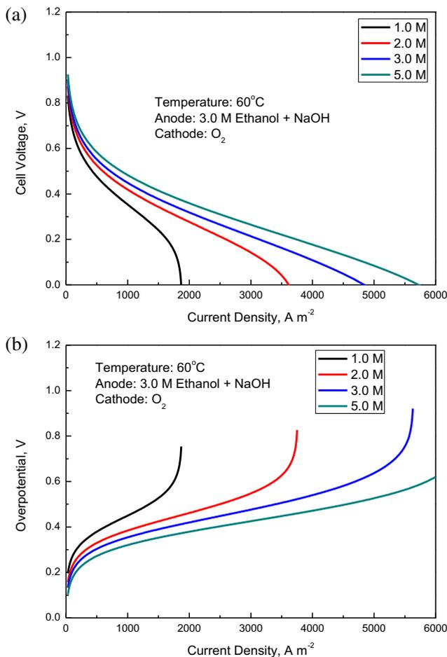
**Fig. 6 – Effect of the alkali concentration on the cell performance. (a) Polarization curves; (b) Anode overpotentials.**
