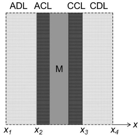
**Fig. 1 – Schematic of an alkaline DEFC and the coordinate system.**
