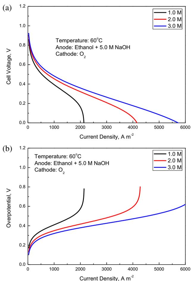
**Fig. 4 – Effect of the ethanol concentration on the cell performance. (a) Polarization curves; (b) Anode overpotentials.**
