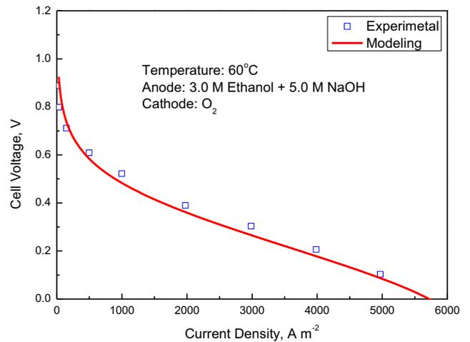
**Fig. 2 – Comparison between the numerical results and experimental data [18].**
