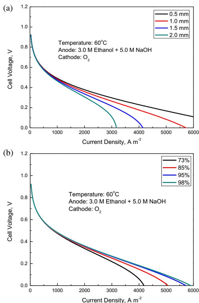
Fig. 10 – Effect of the anode DL parameters on the cell performance. (a) Thickness; (b) Porosity.
