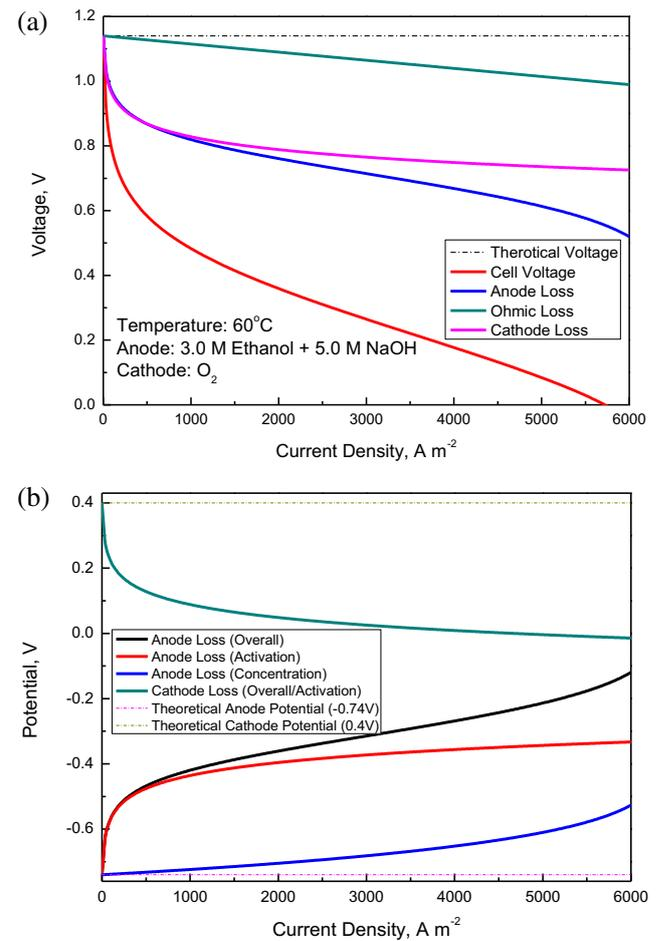
Fig. 3 – Specific loss with the current density. (a) Voltage loss; (b) potential loss.
