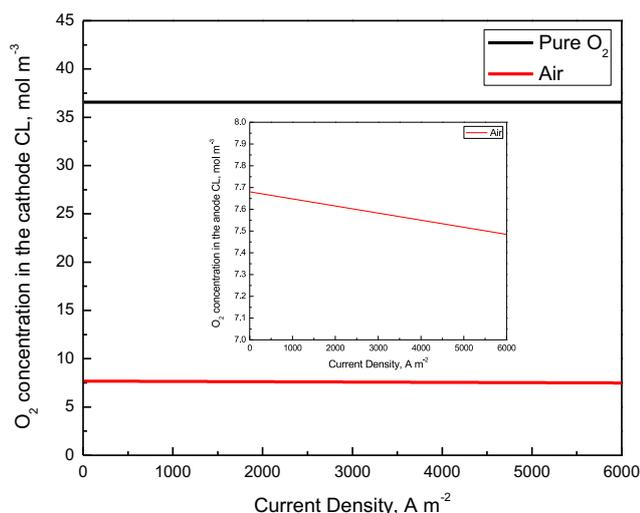
Fig. 9 – The oxygen concentration in the cathode CL.
