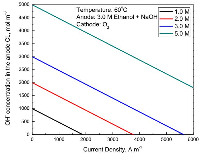
**Fig. 7 – The alkali concentration in the anode CL.**
