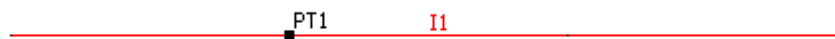
Figure 5.23 Two domains in COMSOL with PT1 the interface of the left and right domain The length of the left domain is 0.001 m and the length of the right is 0.002 m
