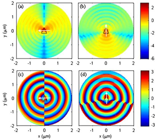
Fig. 2. (Color online) (a) Logarithmic electric energy density distribution at the air/silver interface with  $x$ - and (b)  $y$ -linearly polarized illuminations. (c) Corresponding phase distribution of longitudinal surface plasmon field with  $x$ - and (d)  $y$ -linearly polarized illuminations. The arrow line indicates the input polarization direction.
