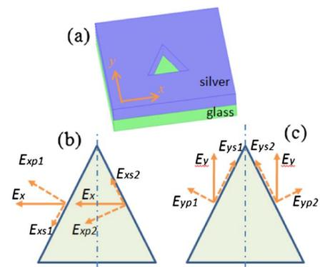
Fig. 1. (Color online) (a) Schematic diagram of an isosceles triangular slot etched into 120-nm-thick silver film. A linearly polarized beam illuminates from the glass substrate side. (b) Explanation of phase mismatch of surface plasmon excitation with  $x$ -linear polarized illumination and (c) phase match with  $y$ -linear polarized illumination.
