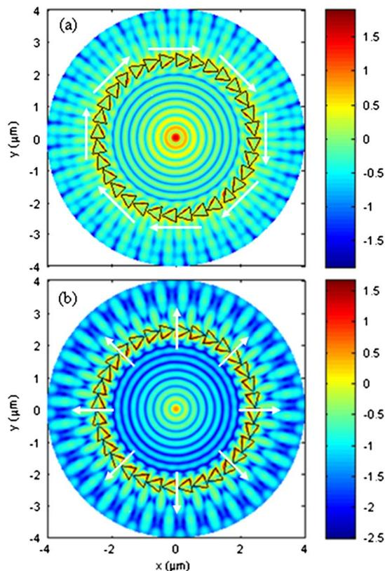
Fig. 4. (Color online) (a) Logarithmic electric energy density distribution at the air/silver interface with 32 isosceles triangles arranged in antisymmetric mode under azimuthally polarized illumination. A highly confined focal spot is obtained at the center. (b) Logarithmic electric energy density distribution of the same structure under radially polarized illumination. A solid spot with lower field enhancement is observed.
