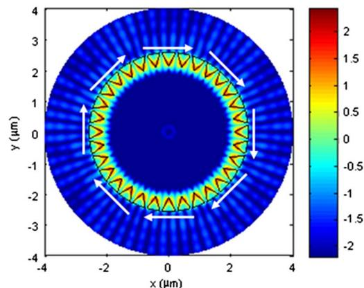
Fig. 5. (Color online) Logarithmic electric energy density distribution with 32 isosceles triangles arranged in symmetric mode under azimuthally polarized illumination.
