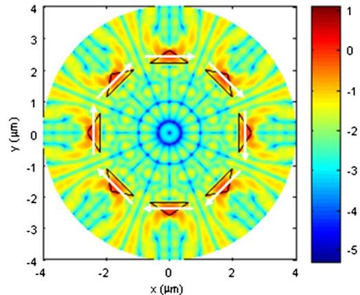
Fig. 3. (Color online) Logarithmic electric energy density distribution at the air/silver interface with eight isosceles triangles arranged in symmetric mode under azimuthally polarized illumination (illustrated by the arrows). Doughnut spot is obtained due to destructive interference of surface plasmons.
