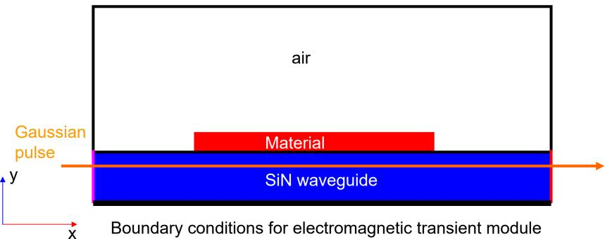
Boundary conditions for electromagnetic transient module
