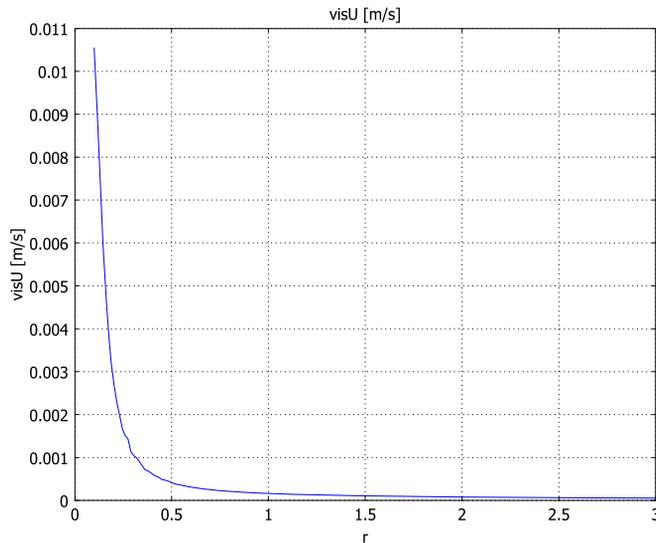
Figure 4: Velocity across the Darcy-Brinkman interface. Cross section along  $z = -0.5$  m from  $r = 0.1$  to  $3.0$  m.
