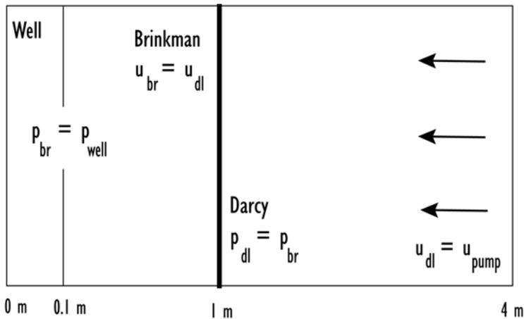
Figure 1: Model geometry showing boundary conditions for coupling Darcy's law ( $1 \text{ m} < r < 4 \text{ m}$ ) and the Brinkman equations ( $0.1 \text{ m} < r < 1 \text{ m}$ ).
