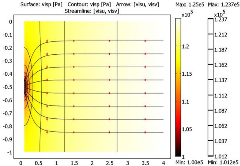
Figure 2: COMSOL Multiphysics solution for Darcy's law ( $1 \text{ m} < r < 4 \text{ m}$ ) and the Brinkman equations ( $0.1 \text{ m} < r < 1 \text{ m}$ ). The results shown are pressure (surface plot and contours) and velocities (streamlines). Note that the vertical axis is expanded.
