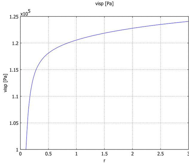
Figure 3: Pressure across the Darcy-Brinkman interface. Cross section along  $z = -0.5$  m from  $r = 0.1$  to  $3.0$  m.
