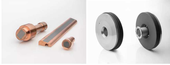
Figure 2. Stationary X-ray anodes made of Cu (left) and rotating X-ray anode made of Mo-alloy with graphite body (right), all with WRe-alloy focal tracks (Plansee SE).
