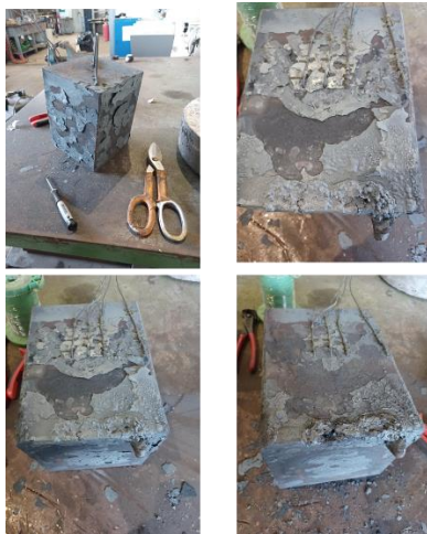
Figure 9. Billet after induction heat treatment in the temperature range from 20°C to 1300°C
