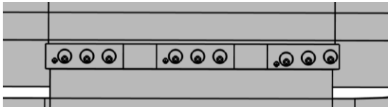
Figure 3. Cables installed in flat formation – Side view.
