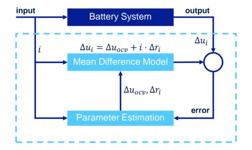
Parameter estimation of \(\Delta u\_{ocv}\) and \(\Delta r\_i\) to minimize error
