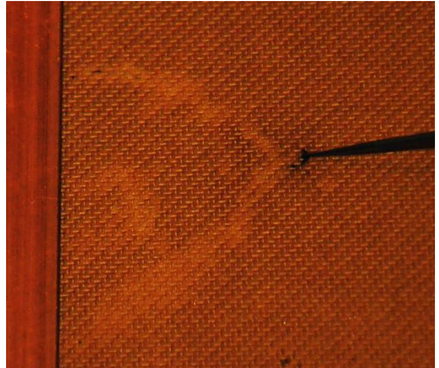
Figure 2: Pressboard surface with white and carbonised marks due to surface discharge experiment
