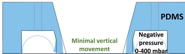
Figure 1: Side view of the optimized structure with minimal vertical movement of the membrane when partial vacuum pressure is applied.
