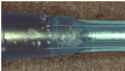
Figure 1. An example of unsuccessful transfer of particles (white) during injection with a hypodermic needle
