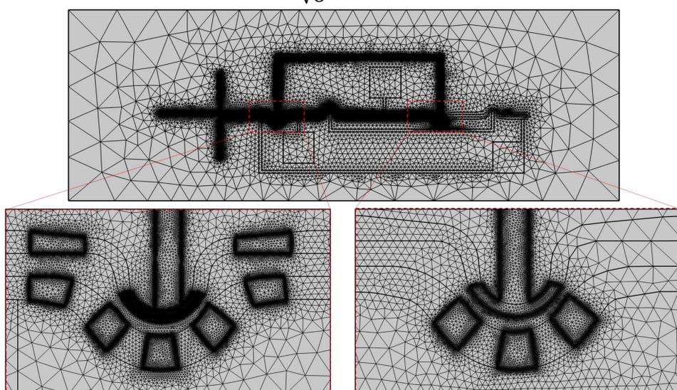
Figure 2. Image of numerical mesh containing approximately 260,000 elements used to resolve the phase field interfaces and subsequent charge accumulation.
