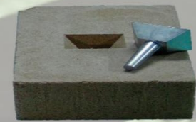
Mould ready for pouring (within one hour)
